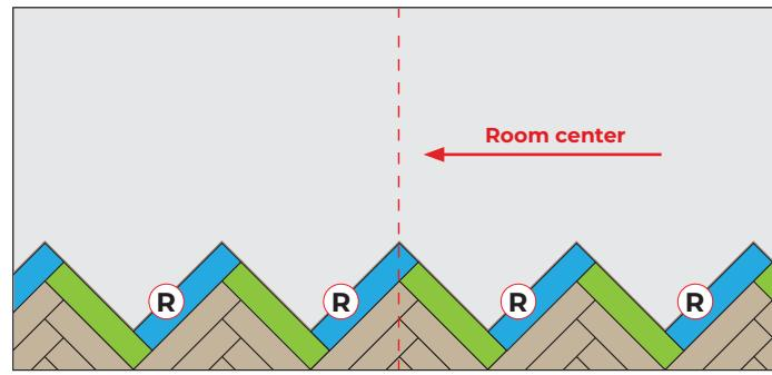
Use the cuttings obtained from the triangles prepared for the starting row to close the spaces left open towards the perimeter walls.
