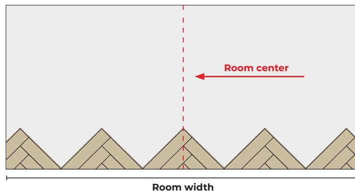
Measure the width of the room where the floor is to be installed and use it to understand how many triangles will be needed to build the first installation row.
