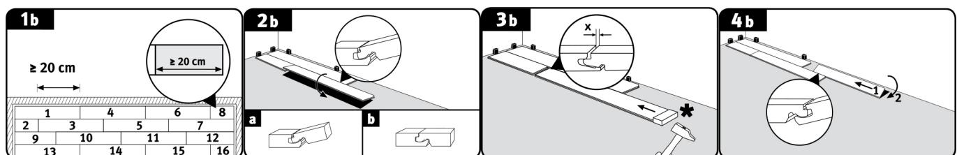
In this angled position, bring the slat 3 as close as possible to the front edge of the slat 2 so that the front male part of the slat 3 is on the milling of the female part of the slat 2 (fig. 3b). Then lock the longitudinal connection by lowering plank 3. Make sure briefly that the front male is not too high compared to the front connection of plank 2 (fig. 3b).
