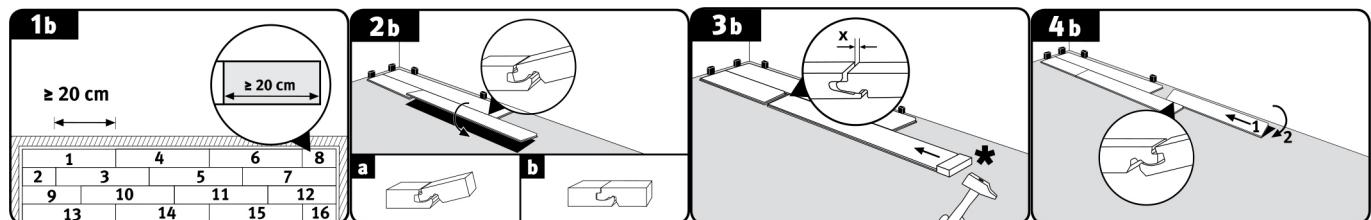
In this angled position, bring the slat 3 as close as possible to the front edge of the slat 2 so that the front male part of the slat 3 is on the milling of the female part of the slat 2 (**fig. 3b**). Then lock the longitudinal connection by lowering plank 3. Make sure briefly that the front male is not too high compared to the front connection of plank 2 (**fig. 3b**).
